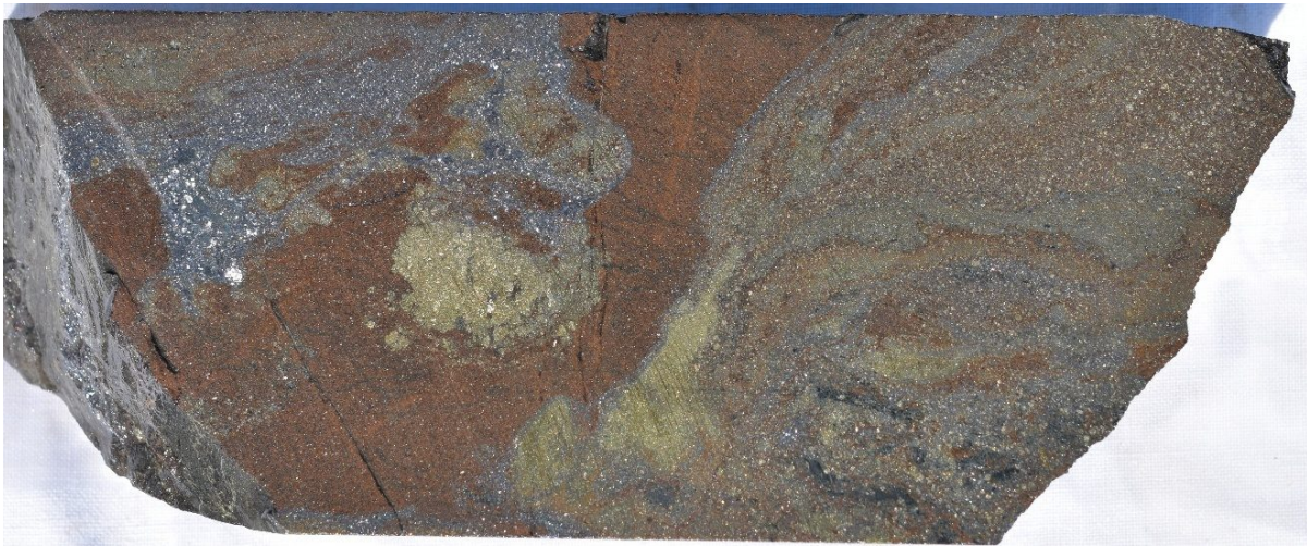
Figure 3: Massive sphalerite + galena + pyrite at 619ft. (188.7m).
