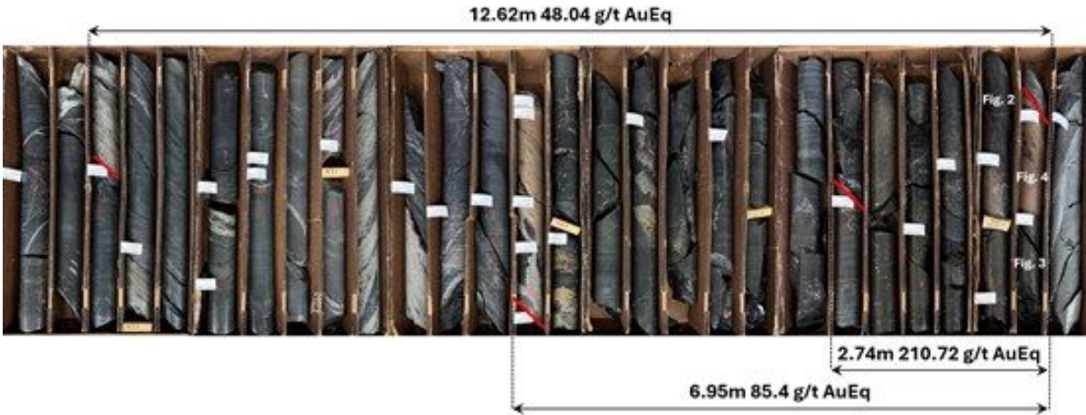
Figure 1: Panoramic photograph showing the nature of mineralization at Silver Hill. Note widespread presence of massive to semi-massive sulfides within a 12.62m interval. Run blocks are in feet.
